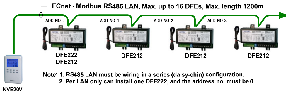
FIG. 1 NVE20V application network architecture diagram
